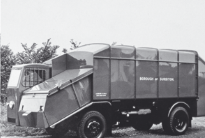
3 - Dennis 'Vulture' collection vehicle – an interesting shaped vehicle in use with its extra compartment in Surbiton (was eagle).
