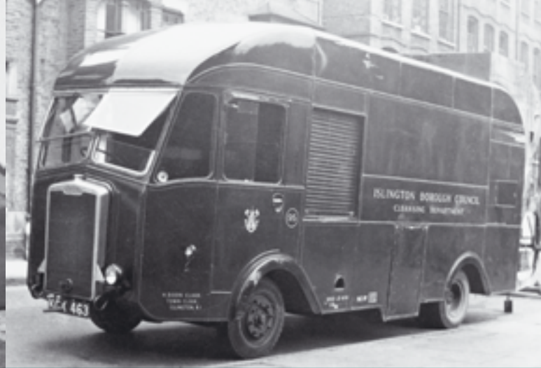
4 - Pagefield 'Paladin' vehicle. While the vehicle is no longer about, 'paladin bins' and versions of them are still in use across the world. The photo also shows the crew using the loading device.
